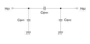
Vertical transfer clock equivalent circuit
